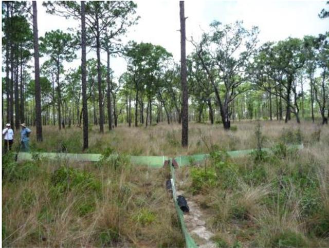
Figure 2. Drift fence with 8-meter arms, funnel traps, and pitfall traps
